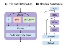
Figure 3: GCN layer (a), using three different propagation rules and a node-wise FC layer. Using residual connections (b) allows a n-layer modular GCN to learn any polynomial function of order n of its constituent operators.
