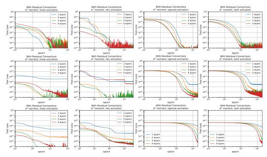
Figure 4: Test loss over number of epochs for learning first (top), second (middle) and third (bottom) order graph moments  $M_p(A) = \sum_j (A^p)_{ij}$ , with varying number of layers and different activation functions. A multi-layer GCN with residual connections is capable of learning the graph moments when the number of layers is at least the target order of the graph moments. The graphs are from our synthetic graph dataset described in Sec. 6.
