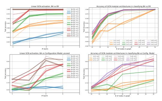
Figure 6: Classify graphs of **Barabasi-Albert** model vs. **Erdos-Renyi** model (top) and **Barabasi-Albert** model vs. **configuration** model (bottom). Left: test accuracy with respect to network depth for different number of nodes (N) and number of units (U). Right: test accuracy with respect to graph size for different number of layers (L) and number of units (U).
